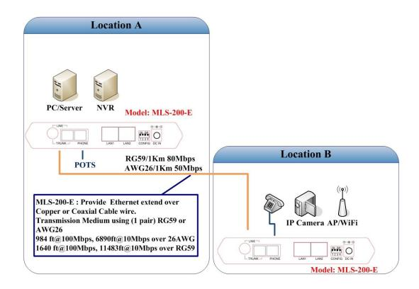
Product Model MLS-200-E, Long Reach Ethernet Convert, 100/100Mbps , 2-Port Ethernet over LRE Bridge (Combo Interface for Copper or Coaxial)
